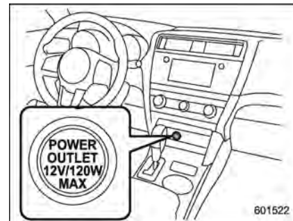
Power outlet below the climate control
