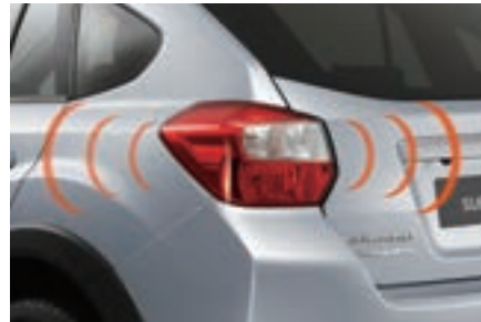
71 Tip blinking and safety hazard kit H705EFJ000 Bi-functional safety item: side indicators blink 4 times and hazard lights are activated during emergency braking.
