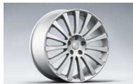
24 Alloy wheel 15-spoke, Crystal silver (19 inch) SECWFG4000 E 8.5"x19" offset 55 PCD 114.3 Tyre size 245/35R19
