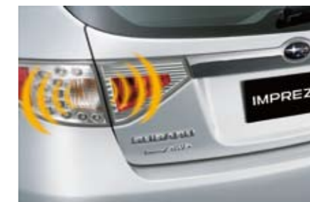
98 Tip blinking & Safety hazard kit SEDAYA8000 E Bi-functional safety item: side indicators blink 4 times and hazard lights are activated during emergency braking.
