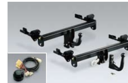
49 Trailer hitch (Detachable, Fixed) See application list W *Maximum towing capacity may vary according to the vehicle specification. Please contact your dealer for details.
