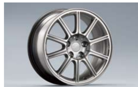
35 Alloy wheel 10-spoke, Platinum silver (17 inch) 28111FE371 W 8"x17" offset 53 PCD 114.3 Tyre size 235/45R17
