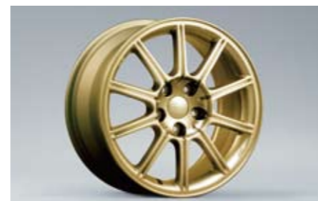
32 Alloy wheel 10-spoke, Gold (17 inch) 28111FE321 W 8"x17" offset 53 PCD 114.3 Tyre size 235/45R17
