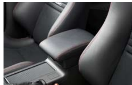
80 | Dual console box J2010FG000JC W Extra storage within existing centre armrest console.
