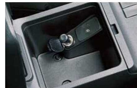
67 Cigarette lighter kit H6710FG000 Changes the accessory socket to a cigarette lighter.
