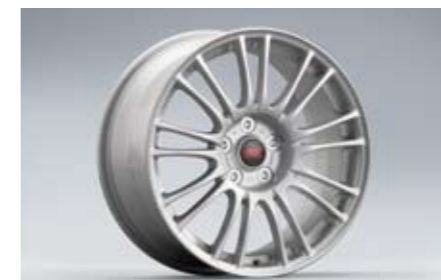
15 Alloy wheel 9-spoke, Silver (18 inch) 28111FG070 8.5"x18" offset 55 PCD 114,3 Tyre size 245/40R18
