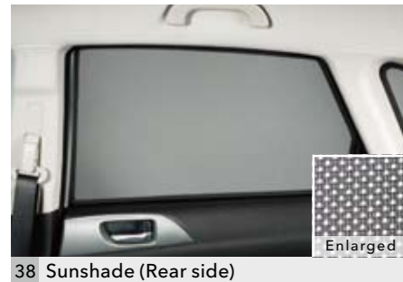
38 Sunshade (Rear side) F505EFG200 Protects from sunshine and darkens your luggage compartment. Mesh type.
