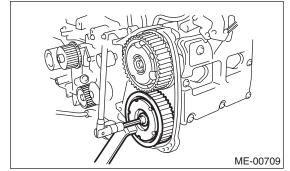
ST 499977500 CAM SPROCKET WRENCH
