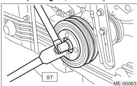
3) Check that the tightening angle of the clamp pulley bolt is a minimum of  $65^{\circ}$ . Perform the following procedure when less than  $65^{\circ}$ .
