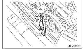
5) Install the V-belts. <Ref. to ME(H4DOTC)-40, INSTALLATION, V-belt.>
