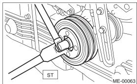
3) Remove the crank pulley.
