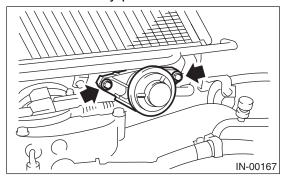
3) Disconnect the air by-pass hoses from air valve.
