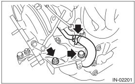
5) Install the joint pipe to turbocharger.
