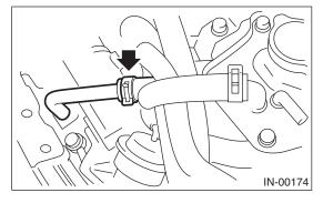
8) Loosen the clamp which secures turbocharger to intake duct.
