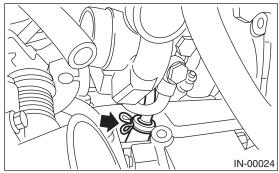
12) Take out the turbocharger from engine compartment.
