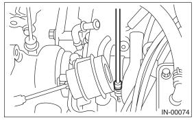
9) Disconnect the engine coolant hoses from pipe, and remove the turbocharger bracket RH.
