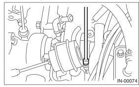
3) Install the oil inlet pipe to turbocharger.
