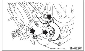
10) Remove the oil inlet pipe from turbocharger.
