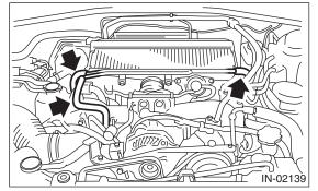
3) Remove the air by-pass valve from intercooler.
