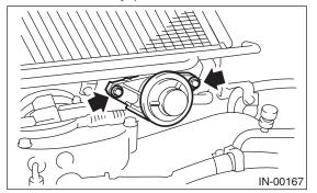
2) Remove the intercooler ducts from intercooler.
