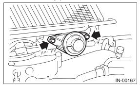
4) Remove the bolts which secure the intercooler to the bracket.
