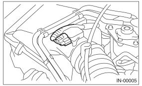
3) Loosen the clamps (A) which connect the air intake boot and the intake duct.
