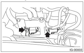
6) Remove the spark plug with a spark plug socket.
