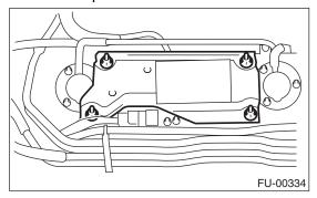
3) Loosen the clip and disconnect the evaporation hose from the fuel cut valve.
