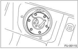
10) Remove the fuel sub level sensor.
