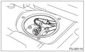
9) Remove the bolts which install fuel sub level sensor on fuel tank.
