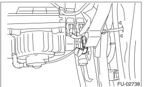
5) Remove the electronic throttle control relay from the mounting bracket.
