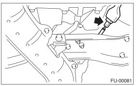
5) Remove the clip by pulling out from the upper side of crossmember.
