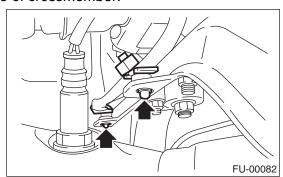
6) Apply spray-type lubricant to the threaded portion of rear oxygen sensor, and leave it for one minute or more.
