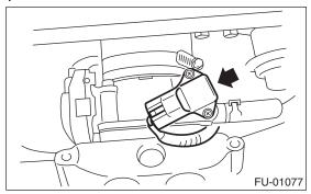
4) Remove the manifold absolute pressure sensor from throttle body.
