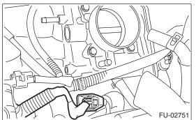
5) Remove the knock sensor from the cylinder block.
