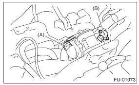
5) Disconnect the engine coolant hoses from throttle body.
