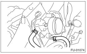
6) Remove the bolts which install throttle body to the intake manifold.
