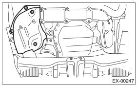
7) Remove the nuts which hold the front exhaust manifold to joint pipe.
