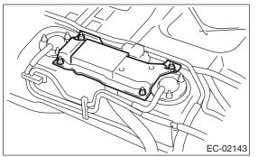
3) Remove the clip and disconnect the hose from the vent valve.
