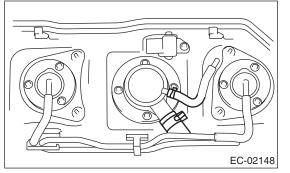
4) Remove the nut and then remove the vent valve.
