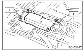
C: INSPECTION Make sure the hoses are not cracked or loose.
