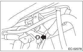
6) Disconnect the connector from the pressure control solenoid valve.
