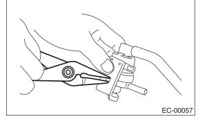
9) Disconnect the hose from the pressure control solenoid valve.
