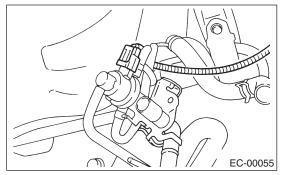
7) Disconnect the two evaporation hoses from the pressure control solenoid valve.
