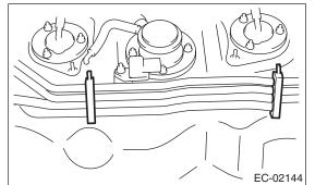
5) Remove the bolt and nut which secures the fuel tank pressure sensor to the bracket.
