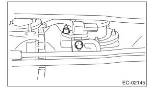
6) Disconnect the pressure hose from the fuel tank pressure sensor.
