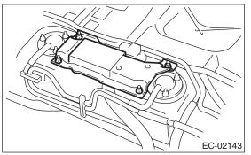
3) Disconnect the connector from the fuel pressure sensor.
