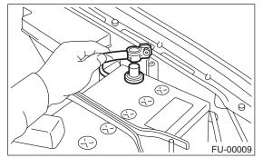
2) Disconnect the connector (A) from secondary air pump.
