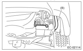
8) Remove the canister from the body.
