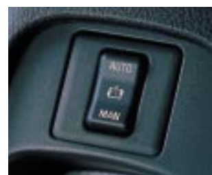
■ Intercooler spray switch
