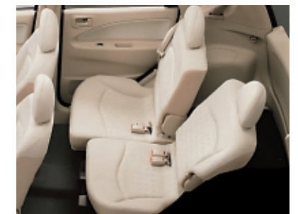
Individual rear seats (each slides and tumbles independently)
