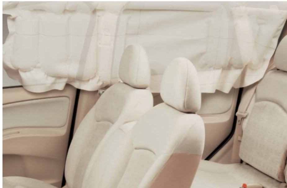
Side curtain SRS* airbag
