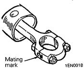
For prevention of wrong installation or reassembly and for ease of operation, put mating marks to the parts where no function is adversely affected.
