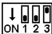
ADJUSTING OF MICROSWITCHES FOR CARS WITH SIEMENS INJECTION AND LAMBDA PROBE, GENERALLY 5 - WIRE BOSCH
