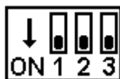
ADJUSTING OF MICROSWITCHES FOR CARS WITH MARELLI INJECTION AND LAMBDA PROBE, GENERALLY 5 - WIRE NTK
